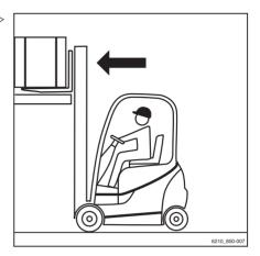
Lift the fork carriage until the load is resting entirely on the fork.
